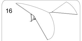
Wing Tissue. Throughout this step, hold the wings in the "down" position, and be sure the wing wires stay all the way back in their tubes. Spread a thin layer of glue on the top of each wing spar and attach the straight leading edge of the wing tissue there. Allow the tissue to center itself naturally as you glue it to the top of the motor stick. Make sure the wing wires are not able to slide forward.
