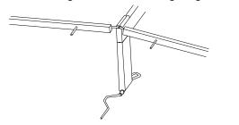
17 Rubber Band. Hold together the ends of the rubber. Tie a knot as shown, forming a large rubber band. Then tie the free ends together to secure. Do not install the rubber band on the model until all glue is completely dry. Then, double the rubber band and hook it onto the motor hooks, with the knot in the back.
